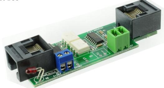
damage the host. The CE-0046S isolates the RS-232 interface from the RS-485 side through an optical isolation barrier rated at over 3,000 volts. Not only does this prevent harmful voltages being coupled through to the RS-232 side but it also isolates the RS-232 ground from the RS-485 "grounds" which otherwise could affect the inherent common-mode voltage rejection, a problem on many balanced networks.
