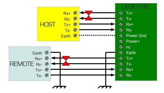
Note: Add 120 ohm termination resistor if equipment is not internally terminated
