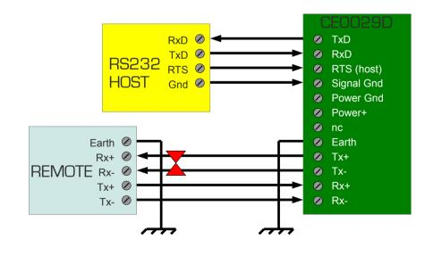
Note: Add 120 ohm termination resistor if equipment is not internally terminated
